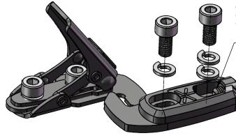
Adjust set screw to desired tension, then tighten hook hardware
