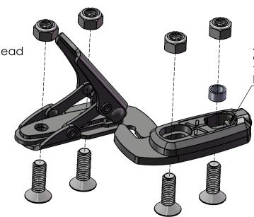
Adjust set screw to desired tension, then tighten hook hardware
